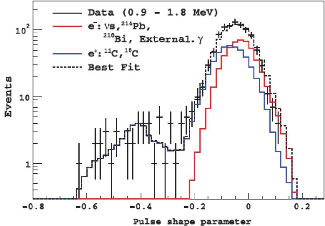
FIG. 2 (color). Experimental distribution of the pulse-shape parameter (black data points). The best-fit distribution (dashed black line) and the corresponding  $e^-$  (solid red line) and  $e^+$  (solid blue line) contributions are also shown.
