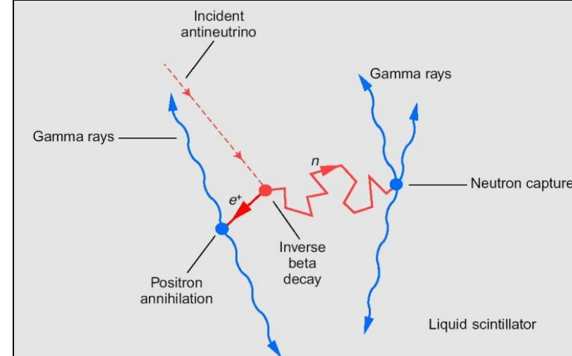
Positron-Gamma (2.2 MeV) delayed coincidence
